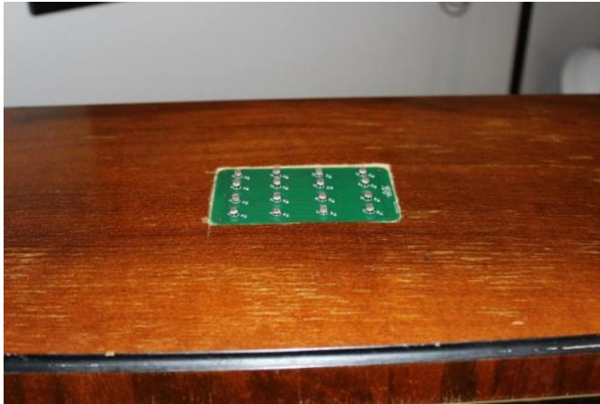
Picture 5. LDR Array installed in cabinet.
